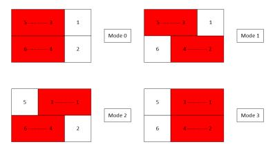
Figure 4: Jumper Settings SPI Mode
